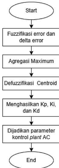
Figure 5. Flowchart of Self-Tuning PID with Fuzzy-Mamdani
