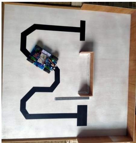
Gambar 22. Pengujian line follower
